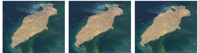
Figure 6. Vertical exaggeration - views of an island at 100%, 200%, and 400% exaggeration
